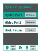
Defines the cycle duration for which the chlorine generation cell runs in polarities 1 and 2 (**Hydro Pol1 and Hydro Pol2**).
