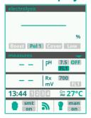
The display of the unit does not show any measured values when the circulation pump is switched off. This also indicates that the control of the water values cannot take place when the circulation pump is stopped.
