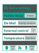
In the menu item "Paddle delay", a time of 0 - 60 sec. can be set to delay the triggering of the flow alarm FL1. This avoids false triggering due to short, system-related response of the external paddle switch or the gas sensor.
